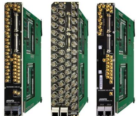
3025EMC with DIN connectors 3025EMC with BNC connectors 3025EMC with XLINK connectors
